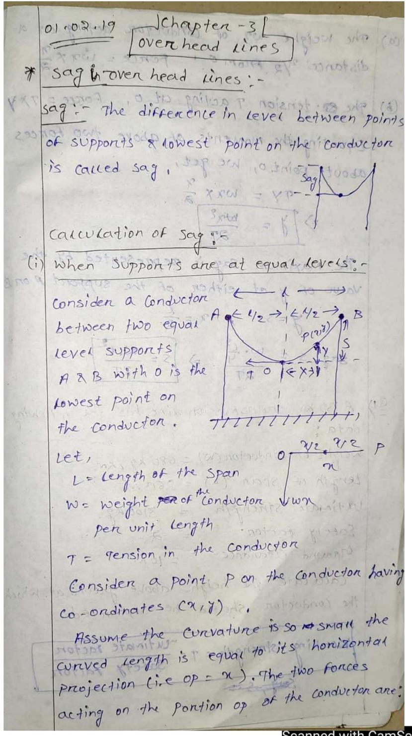
(a) The weight wa of conductor acting at a distance my from o : Fonce = wax 7 The se tension Tacting at o, Force = Try Equating the moments of above two fonces about point o, we get, so bosses à TY = wxx = The Maximum Say is represented by the Value of y at either of the support A on B sag, s = w. L2 => s = w. L2 | s = w. L2 | A 132 KV transmission line has the following weight of conductor (W) = 680 kg/km Length of Span (1) = 260 m
