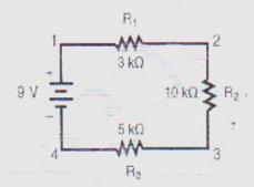
Find the current I passing through and the voltage across each of the resistors in the above circuit.
