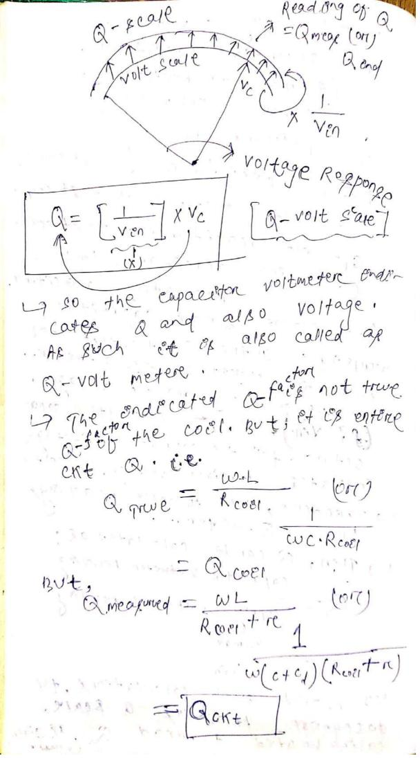
The Repulting distrerence between the measured and true a is error en a - me asurcement. Ererore = Qmeay - Qrove % Erenor = amegy - afring X200%. Atrue
