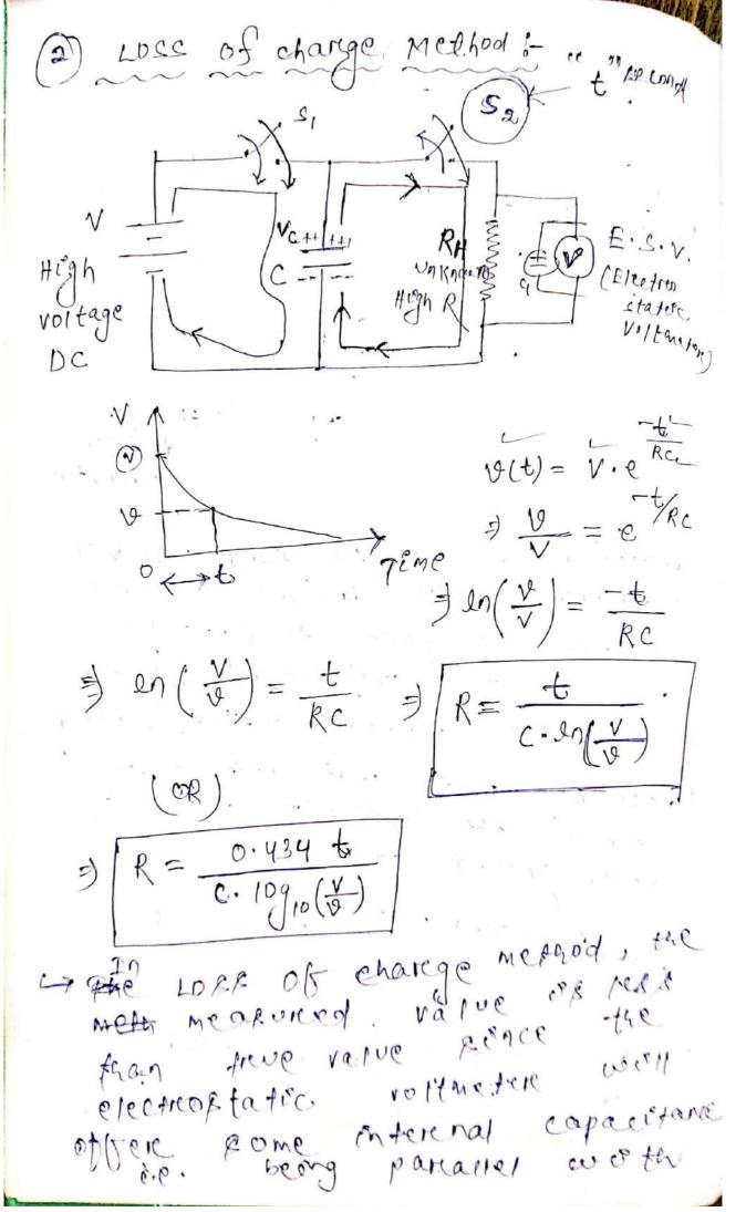
actual capace tance so that met capacitance value oucell increase and R measured (R) decreases. 17 The loss of charge method isk measure-best suctable for the measure-ment of insulation resistance in case of underground cables. € E7. 0157 = € Q. E7. 21TM X1= €0'Q =) == Q == Reoin => (Eo din)
