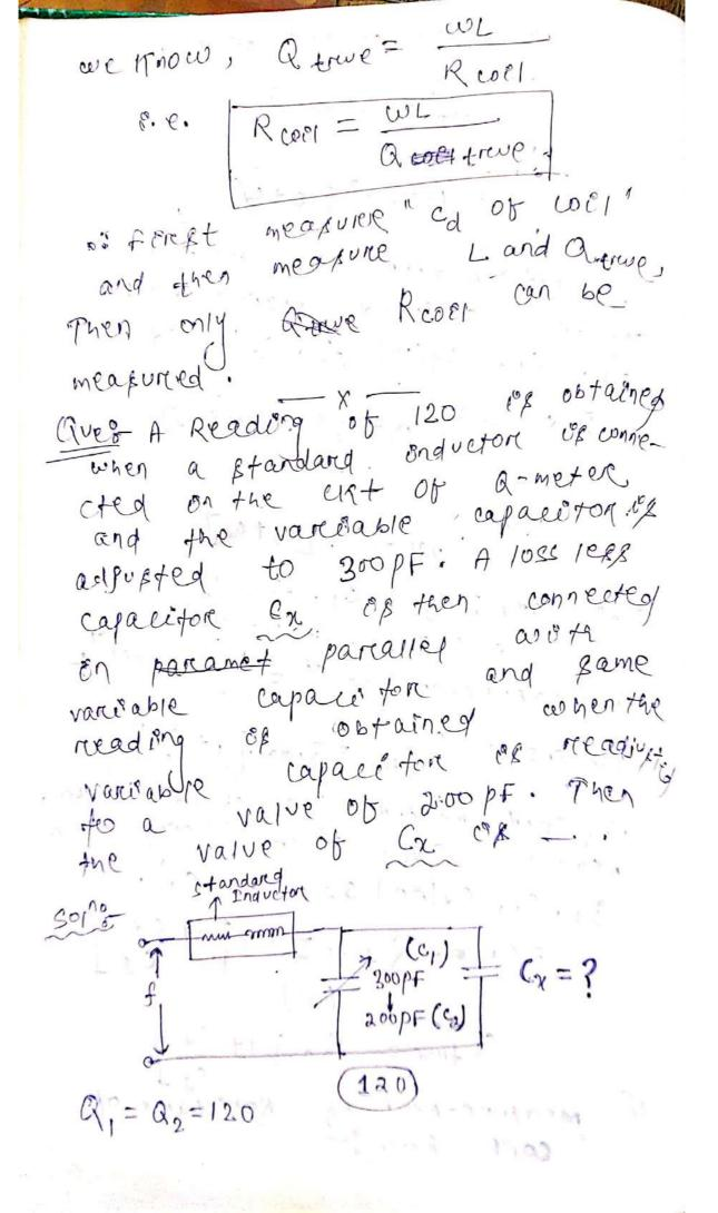
= wo. C. C. Rcoel = w. (catex) Rcoel > CI=Ca+cx =) [Cx = C, -C2 ] unknown capacin-= 300pf-200pf Q-meter. = Tropf Ques A coil of feated with a of the coil of found to be \$20pf. Resonance has occurred at a freeguency of 106 rad , with a capacity of 9.18 nF. what is the inductance of the cool ? 5012. W=106 rad, Cd= 620 PF C=9.18 NF 1= 12TTf)2(c+Cd) = 102. (c+Cd) = (106)2 [9.18nf+820pf) 1200 MH an open the reading of a voltmeter coel the roll of the actor
