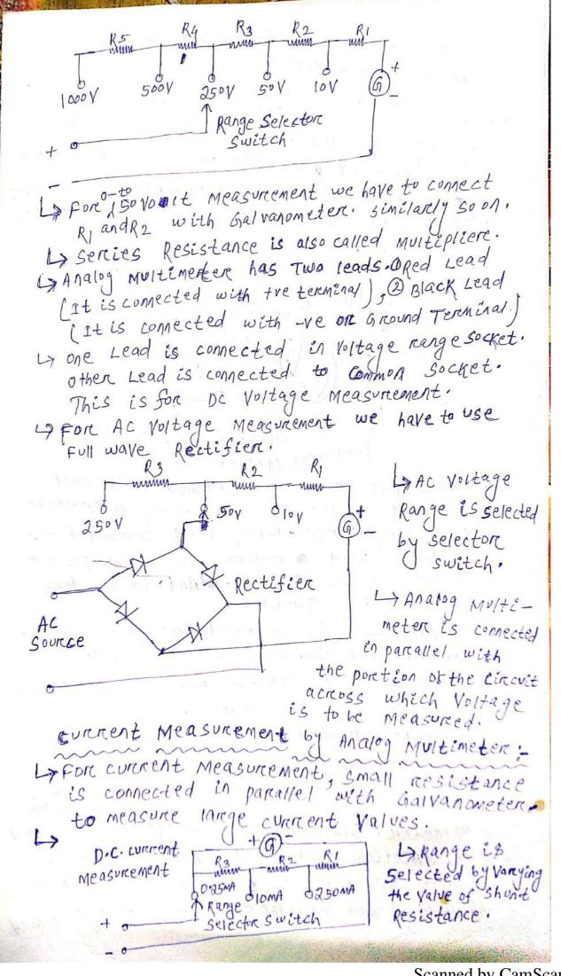
L) Multimeter is connected in series with the branch in which current is to be measured.
