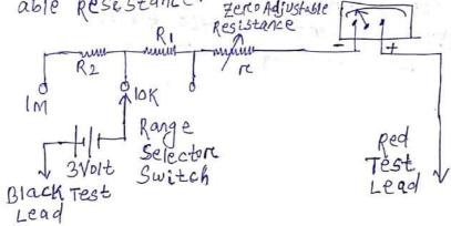
Lafixed Resistances limit the current with in the deserred range. Variable resistance is used for Zero I adjustment in the pointere. scale is ealibrated interems of resistance.
