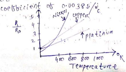
Here a Approximations O Linear Approximation which is used bore short range of temperature @ Quadratic Approximation used for large range of temperature. In Lineare Approximation
