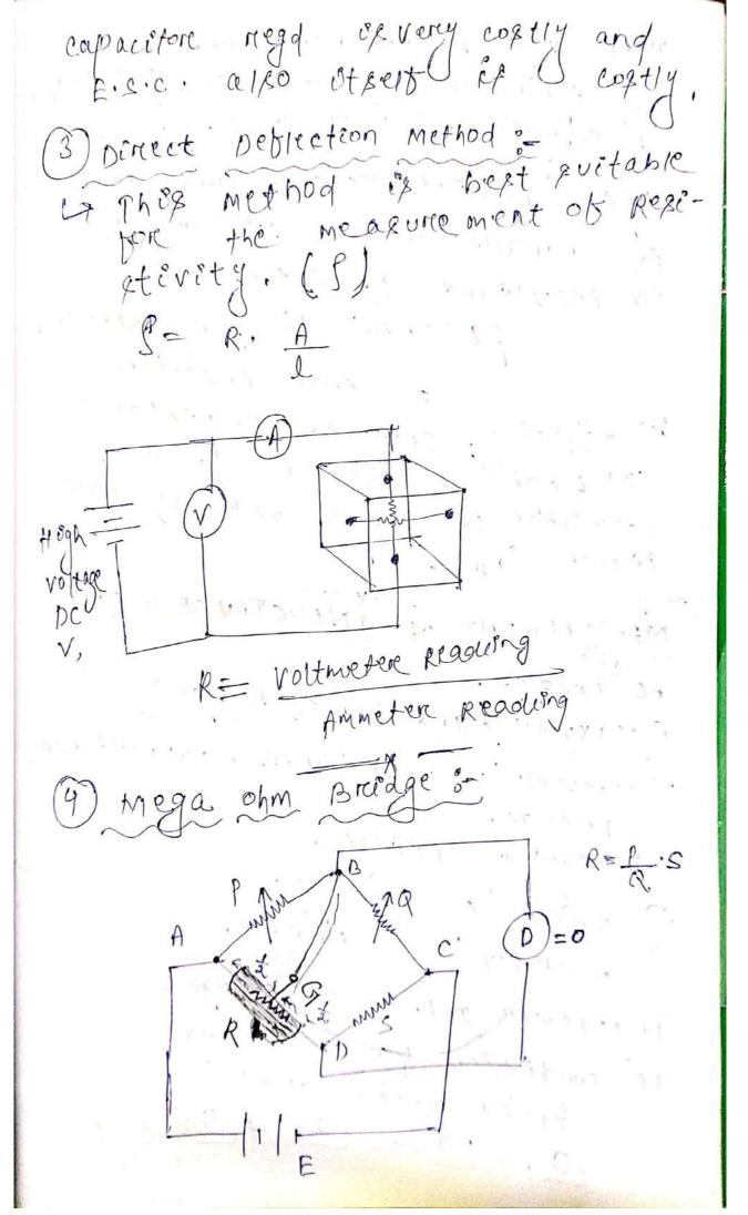
Here High Resistance connected. Here High reminal connected to B' terems
