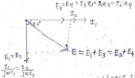
Ly To measure temperateur capacitance ob imperible capacitor (ore) Monider l'imperible capacitor we use modified De-sauty's aridge.
