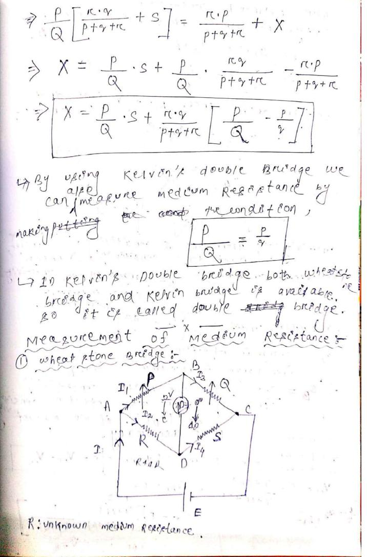
under Balanced condition, voltage drop aeroex AB = voltage drop aeroxx > 1.P= 12.R  $\Rightarrow \frac{T_1}{T_2} = \frac{R}{p}$ voltage drop? aeross BC = voitage drop aeross = ) I, Q = Iy S 3 R= P There are a sensitivity, in wheat those bridge,
