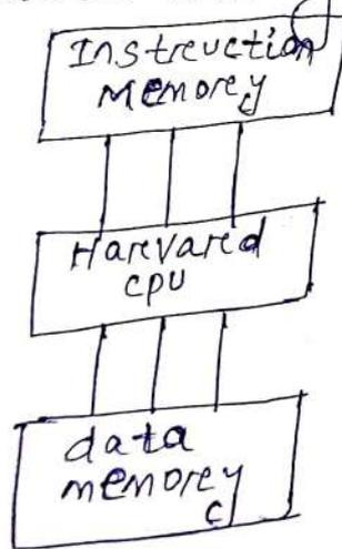
↳ In von-Neuman Architecture, 2 set of clock cycles required. 1 cycle for data fetch, and 1 cycle for instruction fetch. Whereas in Harvard Architecture single set of clock cycle is sufficient.
