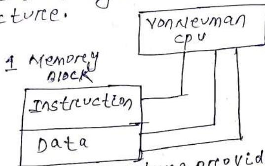
All the buses i.e. Address bus, Data bus, control bus are accessing one memory block in von Neuman Architecture.
