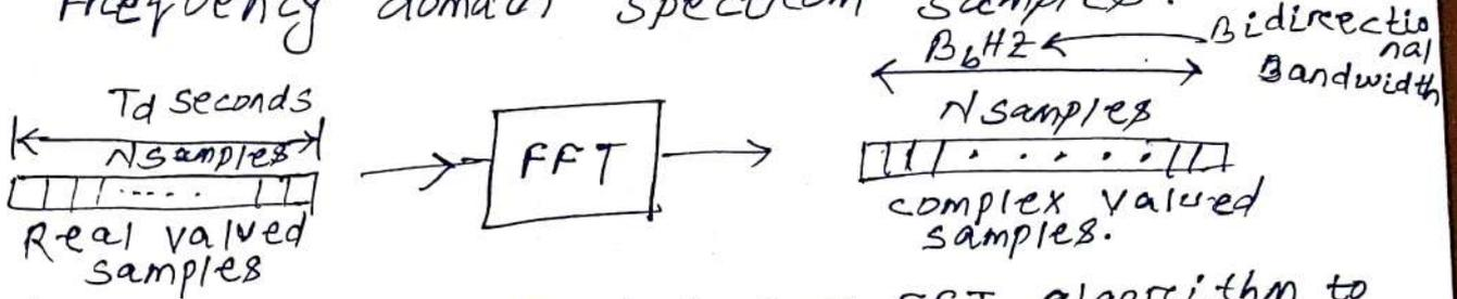
↳  $N$  must be a power of 2 for FFT algorithm to be truly "fast".
